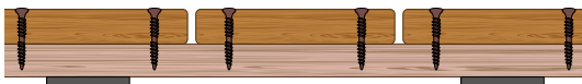
IT-3 Itauba (21x120 mm) installation with visible screws Itauba 21x120 mm posé à visser
