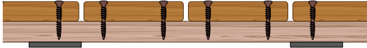
IT-1 Itauba 19x90 mm installation with visible screws Itauba 19x90 mm posé à visser
